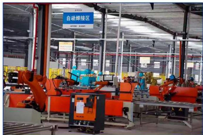
- Fully automatic welding line -
